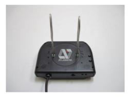
2) Pour distilled water into the one and a half pint Mason jar. Do not fill the Mason jar beyond one inch below the top of the Mason jar. Make sure your CSG-ULTRA is turned off (On/Off switch in the center position). Place the CSG-ULTRA with the silver wires on to the Mason jar as shown below.
