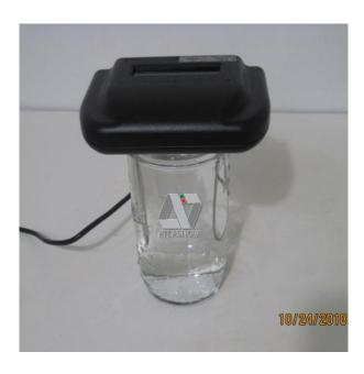
Make sure that none of the silver wires are touching any part of the Mason jar where the water is present. The silver wires should be as far apart as possible
