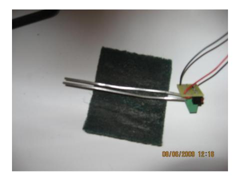
Remove the generator from the water and clean the silver wire with a green scouring pad supplied. Two or three swipes should be sufficient.
