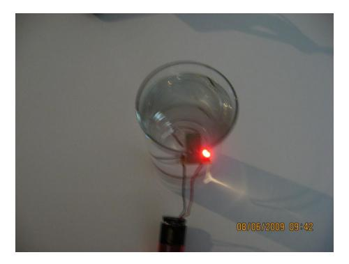
It is now a bit more than two hours later and we can see that the LED is glowing much brighter, indicating that we are running a much higher current than when we started. This indicates that we have generated enough ions to increase the conductivity of the water.
