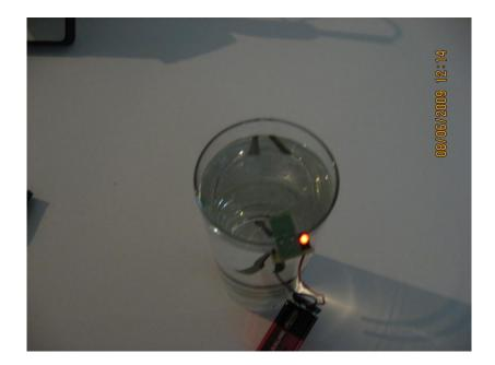
We are now five hours into the process and we can see that the LED is once again at full brightness. At this time, we will once again do the finger test. We observe that the LED's brightness remains the same when we press on the generator. This means that we have achieved well over 10 PPM strength of colloidal silver. Please note that your process could be less than 5 hours depending on the quality of your distilled water.
