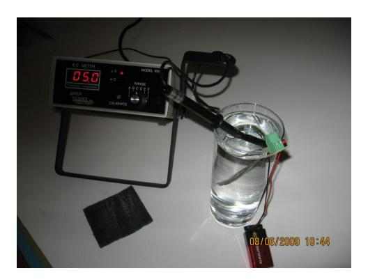
We are now 3 hours into the process, our conductivity meter reads 5 PPM, and we continue the process.
