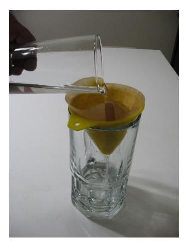
Filter the colloidal silver to remove any large particles that may have formed. A coffee maker filter of the unbleached variety is perfect for this.
