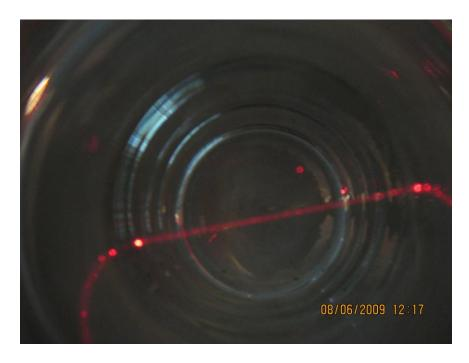
We now use our red laser pointer included with the kit to confirm the fact that we have made actual particles as well as the ions that are measured by an electrical conductivity meter. If we include the particles in our measurement, which are not shown in conductivity, the true PPM would be 17 to 18 in parts per 1,000,000.
