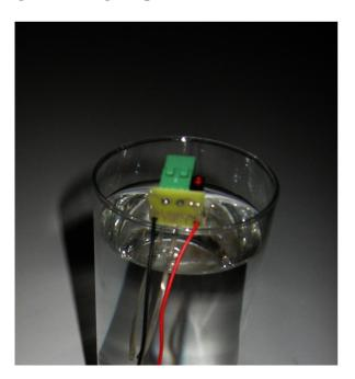
In this picture we can see that the LED is much less bright after we have moved the position of the silver wires.
