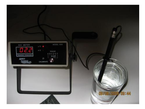
This is confirmed by measuring the PPM of the water in the glass. It reads slightly over two PPM. So we continue the process.
