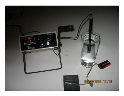
We confirm this with the use of our electrical conductivity meter. It reads 15.1 PPM. Please note that the reading will vary depending on the quality of your distilled water. We are now finished with the process of making our colloidal silver.
