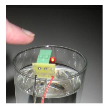
To check if we are done with the process, place your finger on the generator and gently move the position of the wires, as shown in the picture above. Observe the change, if any, in the brightness of the LED. If the LED dims noticeably when we moved the wires in the water, we are not finished.
