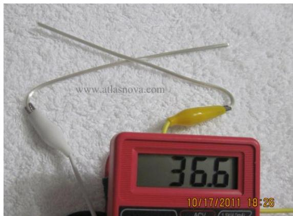
When you put the two silver wires together, this causes the full voltage to flow through the resistor and the meter will read approximately thirty six volts, which happens to be four times nine.
