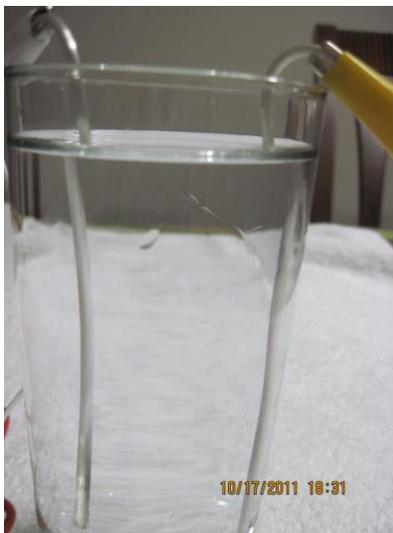
Place the silver wires at opposite ends of the glass containing the distilled water as shown. Make sure that the silver wires are not touching each another. We also do not want any of the silver wire that is immersed in the distilled water to touch the glass itself.
