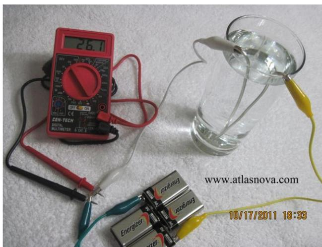
In order to speed up the process you can move the silver wires closer together so that you may generate ions more quickly. The more ions in the water, the higher the conductivity of the water and this allows more current to flow.
