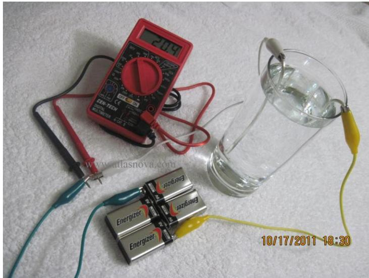
As you can see, the voltage that is being dropped across the resistor is 20.4 volts. The reading of 20.4 volts indicates that the distilled water in this case is not of the same quality as used in the picture below. If this is as good water as you can get, it is still okay to use for making colloidal silver.
