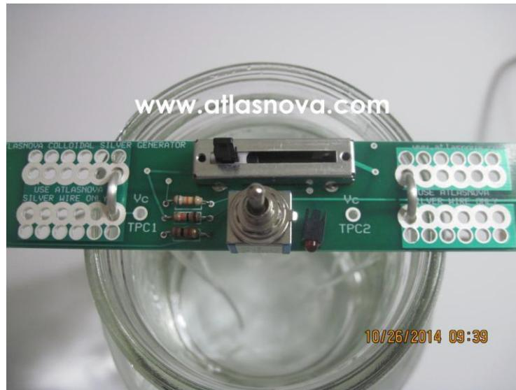
Place the printed circuit board (generator) with the silver wires on to the jar. Make sure that none of the silver wires are touching any part of the jar where water is present. The silver wires should be as far apart as possible.
