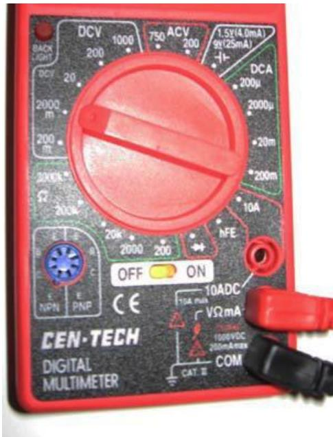
Plug the test leads into the Digital Multimeter at the two lower sockets on the meter. The top socket is not used. It is only there for measuring very high amperage.
