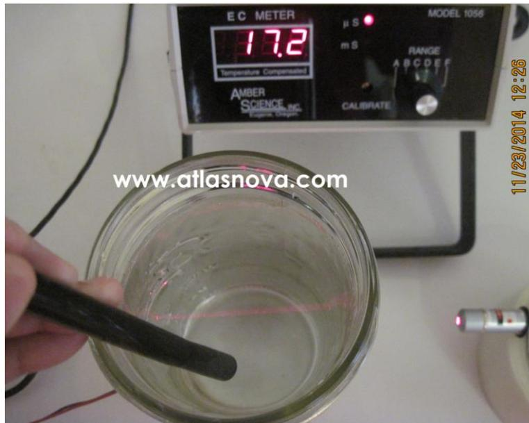
In this picture we have submerged the probe of our Amber Electronic Conductivity Meter to measure the value of conductivity in Microsiemens. This is the same value for the PPM (parts per million) of the ionic part of our colloidal silver. As you can see in our picture, our PPM reads 17.2. Please note that the PPM reading will vary depending on the quality of your distilled water.
