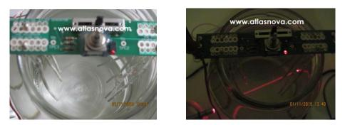
The red laser beam indicates that we have made particulate silver as well as ionic. As you can see by this picture, we have a nice strong red beam even in normal indoor room light. The water itself is still crystal clear. This means that we have avoided making overly large particles.
