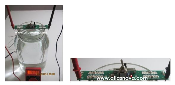
The position of the toggle switch points to the set of wires that will be the anode. By moving the toggle switch all the way to the left, the silver wires that were the anode will now serve as the cathode.
