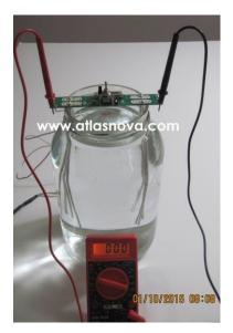
Put the two test leads into the two outer test points on the generator as shown. The meter should read zero volts.
