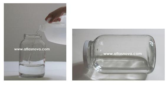
The one-gallon jar that is supplied will be clean when you receive it. However, a good idea would be to fill it half full of distilled water. Replace the cap tightly and give it a good deal of motion so that any dust particles that may have entered will now be in the water.
