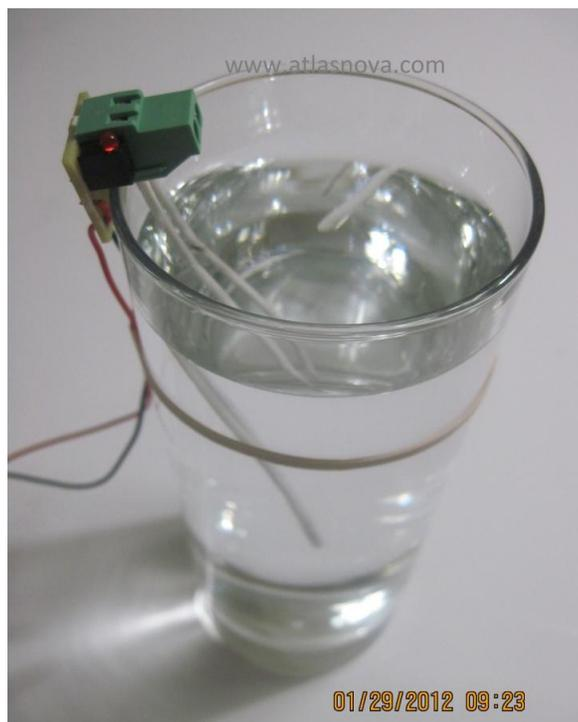
Slide the rubber band onto the glass to make sure that the silver wires are not touching the glass itself. This is to hold the silver wires in the center of the solution. Plug the universal power supply to the power outlet.
