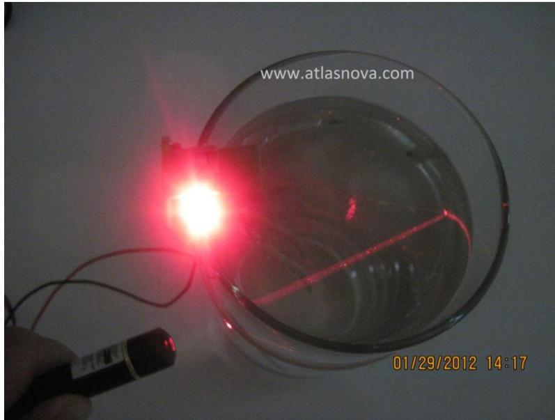
We now use our red laser pointer included with the kit to confirm the fact that we have made actual particles as well as the ions. With the lights off, you can see the red beam created by the laser pointer being scattered by the small particles of silver.
