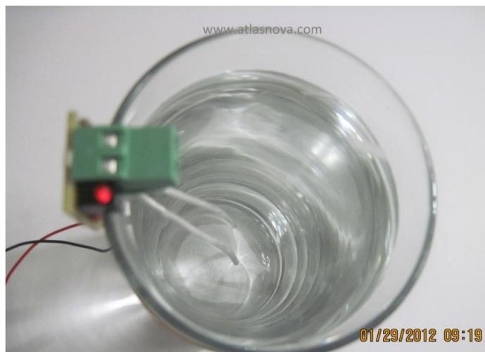
Place the generator on the rim of the glass as shown in the picture. Make sure that the silver wires are not touching each other. Position the printed circuit board (generator) on the rim of the glass in such a way that the ends of the silver wires in the water are near the center of the water, and keep the silver wires at least 1 inch away from any glass surface in the water. Also, make sure that any part of the generator (printed circuit board) is not touching the water.
