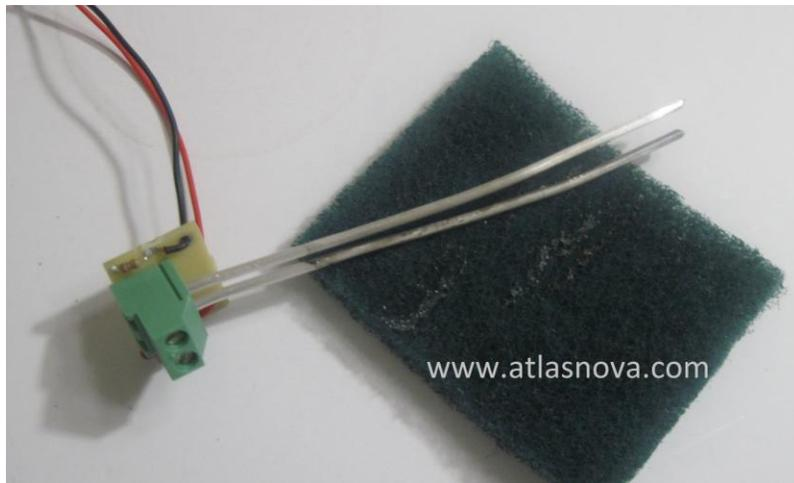
We are now finished with the process of making colloidal silver. Unplug the universal power supply, remove the generator from the water and clean the silver wires with the supplied scrubbing pad. Two or three swipes should suffice.
